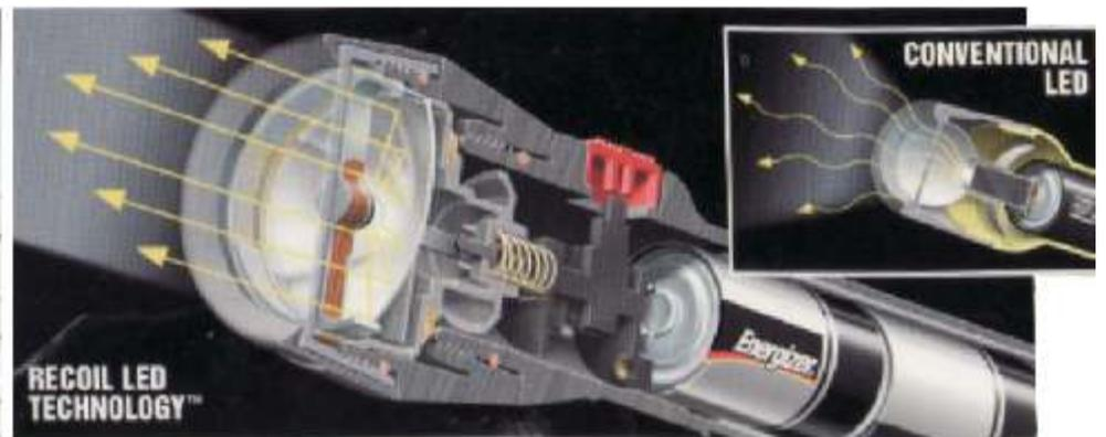
Conventional incandescent and LED torches shine light imperfectly forward with scattered peripheral light as not all light hits the reflector before being projected. The Recoil LED Technology for torches focuses all of the light backwards into the reflector. A modified parabolic reflector then captures 100 percent of the light and reflects it forward.
